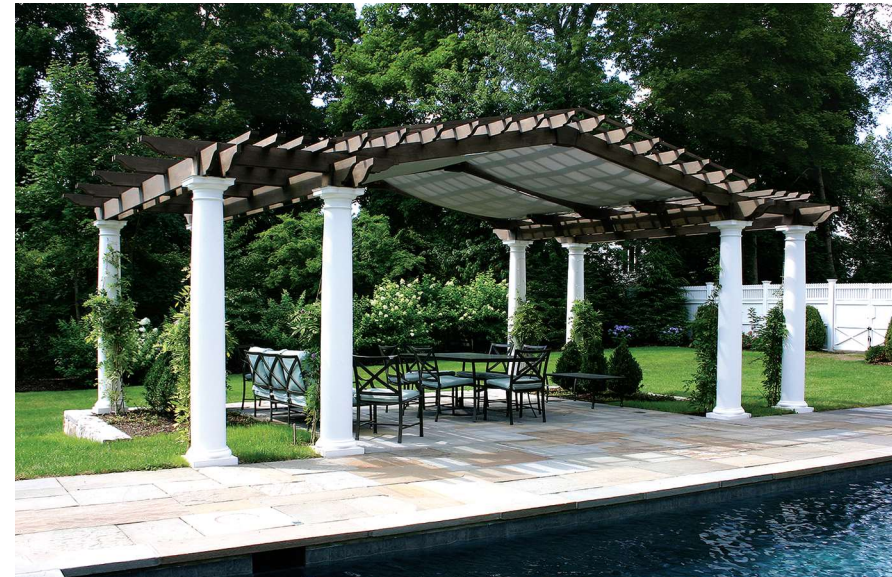
With the cedar components stained a dark brown, this structure was designed to complement a large, formal mid-nineteenth century home. The central peaked area of the structure incorporates a shade cloth, that is swagged over aluminum pipes to facilitate easy removal for the off-season. The peaked structure allows for large, unsupported spans without using extra large beams.
