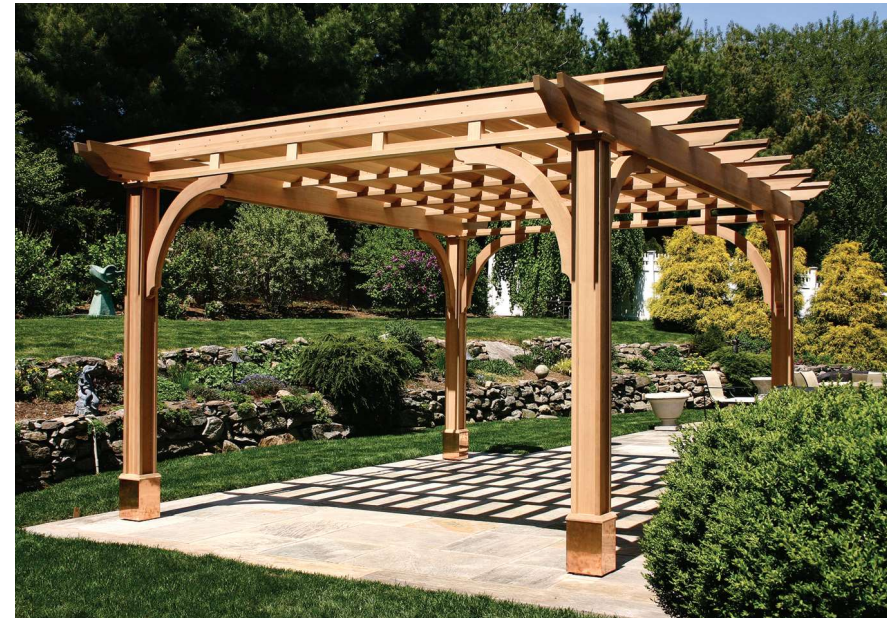
A unique pergola, this large structure uses a combination of louvers and T rafters, with shade cloth installed in the hottest months, to establish a cool area in a very warm back yard. The posts are 7 1/8" x 7 1/8" with a subtle corner bead. The plinth bases, which conceal substantial stainless steel brackets, are covered in copper flashing. Large curved brackets, 3 1/2" thick, add stability while lending softness to the geometry of the design.
